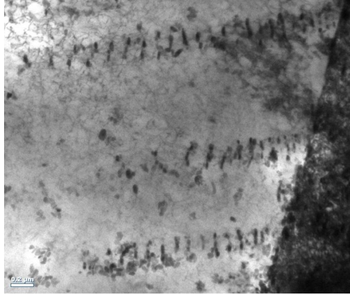
Figure 4.17 TEM micrograph of Haynes 230 deformed at 800 °C and 10^{-3} \text{ s}^{-1} . Precipitates align to form rows at positions previously occupied by dislocations.
