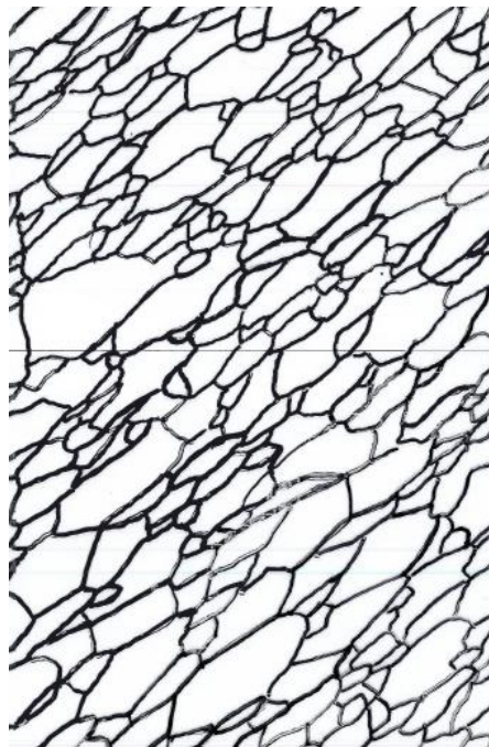
Figure A.2 Transparency used to calculate grain size of Inconel 617 at 800 °C
